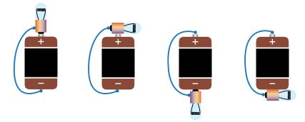
As students work, circulate around the room, helping students focus their attention on determining the various critical contact points on the battery and bulb. Students will most likely be familiar with the two different ends (+ / -) of their batteries but may not carefully observe the contact points involved on the light bulb (connections must be made to the side and base of the bulb). Remind students to record all their attempts and note these contact points.
