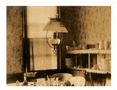
This photo from the Maine State Museum shows a wick style kerosene oil-ceiling lamp from a Maine kitchen around the turn of the 19th century. The small, white fuel tank houses the oil, which is sometimes called paraffin. A cotton wick is partially submerged in the oil. Once the top of the wick is lit, a yellowish flame is produced.
