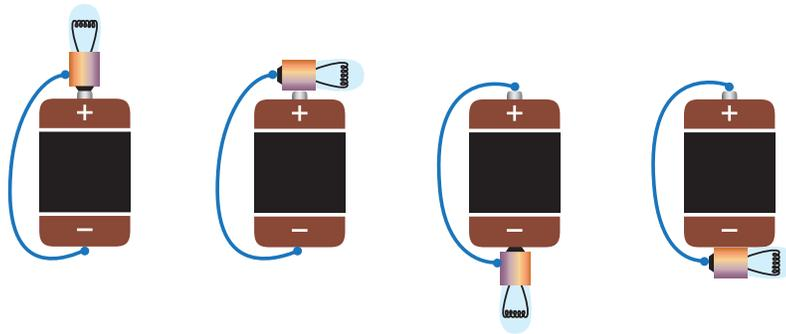
As students work, circulate around the room, helping students focus their attention on determining the various critical contact points on the battery and bulb. Students will most likely be familiar with the two different ends (+ / -) of their batteries but may not carefully observe the contact points involved on the light bulb (connections must be made to the side and base of the bulb). Remind students to record all their attempts and note these contact points.
