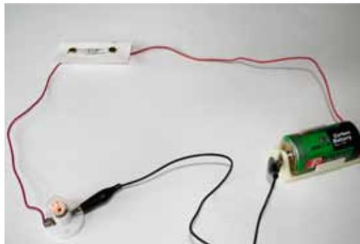
**Note:** Some students may hold naïve ideas about how the circuit works even after building one successfully. They may think that each wire brings electrical energy from the battery up to the light bulb rather than electrical energy traveling in one direction through the wire “loop.” Or they may think one wire is active and one is not. Use their thinking to guide your questioning and discussion.
